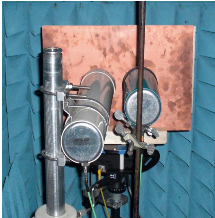
Figure 5.16 - Measurement on flat metal sheet.
